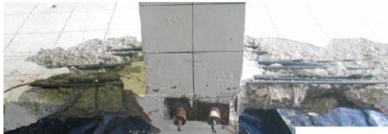
Figure 5.2: Punching failure for PT connection without shear reinforcement with significant drop in floor slab – major repair required [Kang , 2006]
